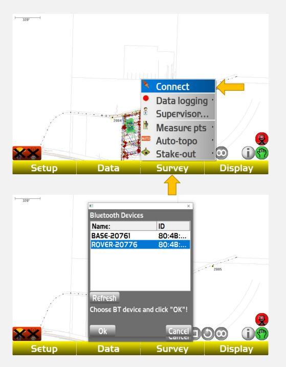
Once you are connected the red box with the rover and antenna icon will turn green. Next, to get your cut/fill to appear, select the survey tab
