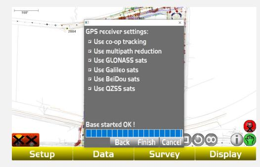
Once Base is successfully launched, you need to connect the rover. Select the Survey tab then click connect
