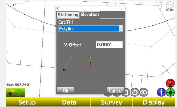
Displayed now is the station, lateral distance to polyline and cut/fill to polyline. In this case, cut to storm invert. The fill in parenthesis is the fill to finish grade.
