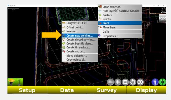
The "Add to layer" menu will appear. Either select an existing layer or create a new layer to place the new linework and click "Ok"
