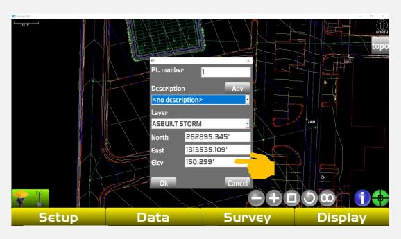
You can now manually change the elevation of that point to your desired starting point elevation, click "Ok"
