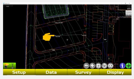
Hold your finger or stylus down on the screen for two seconds until the quick menu appears
