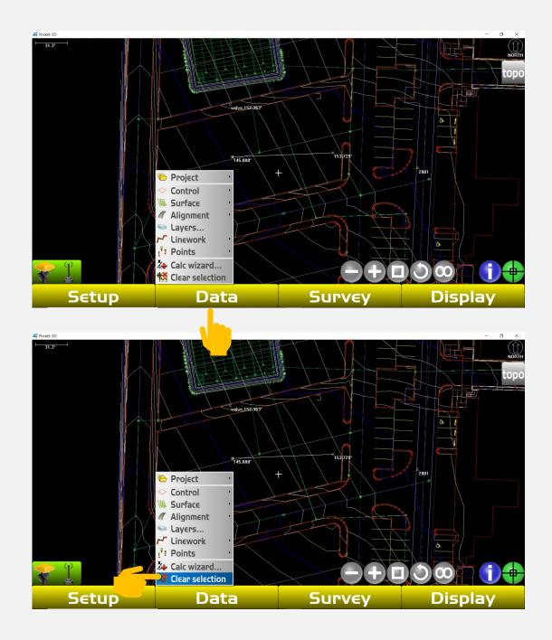
Highlight the end point by either dragging a box around it or simple tapping it with your finger or stylus. Once it is highlighted hold finger or stylus down anywhere on the screen for two seconds. The quick menu will appear
